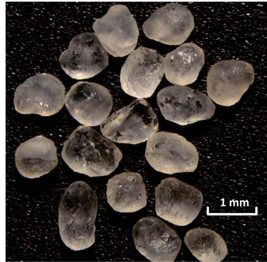
FIG. 5 Optical microscopic image of Ottawa 20-30 sand grains.
